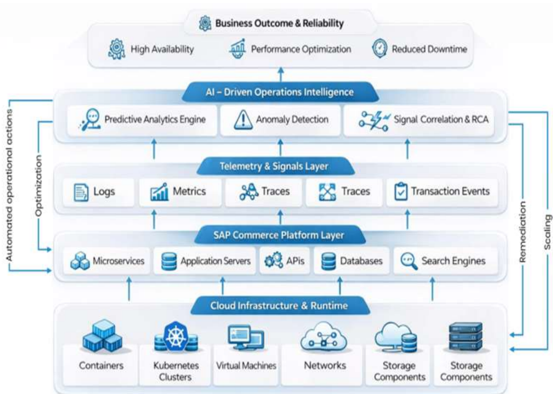
Figure 1: AI-Driven Cloud and SAP Commerce Platform Architecture for Automated Operations and Telemetry”
